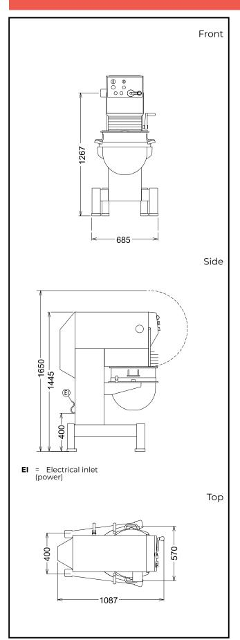
Electric 220-240/380-415 V/3 ph/50 Supply voltage: Electrical power max: 1.54 kW **Total Watts:** 1.54 kW Capacity: ISO 9001; ISO 14001 kg/ Performance (up to): Cycle Capacity: 60 litres Key Information: External dimensions, 685 mm Width: External dimensions, Depth: 1087 mm External dimensions, Height: 1445 mm
